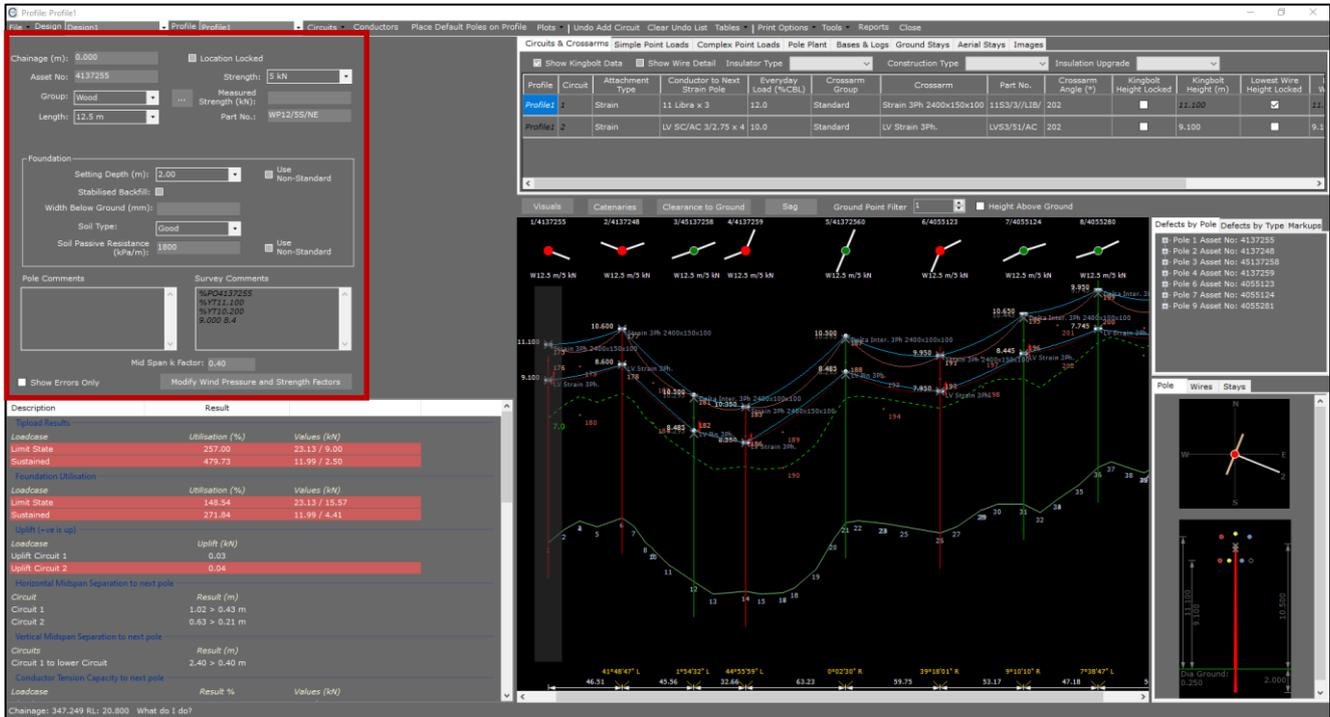
66. A summary of the results on each pole can be viewed by clicking the pole of interest in the profile view (indicated by the grey transparent highlighting). The results are then listed on the left-hand side under the pole attributes
